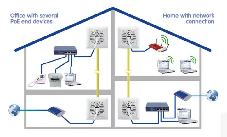
Mx2wire+ converts standard 2-wire cabling into a PoE network connection.
