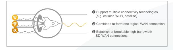
**Unbreakable connectivity** - SpeedFusion Hot Failover maintains secure tunnels over all available WAN links to keep the network up and running when a connection drops out. If a WAN link fails, SpeedFusion instantly routes traffic to a working tunnel for uninterrupted VoIP sessions.
