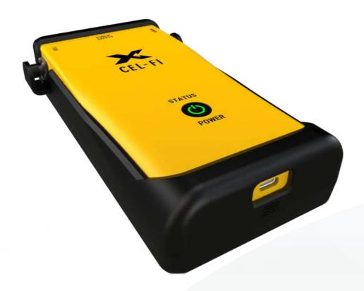
The COMPASS XR scanning receiver is the complete solution to enable integrators to install and optimise CEL-FI cellular and SHIELD public safety coverage systems. A convenient tool in a lightweight and portable package, it can be used globally to deploy and verify multiple technologies, including 5G New Radio networks in sub-6 GHz spectrum, LTE, CBRS, and LMR public safety coverage.
